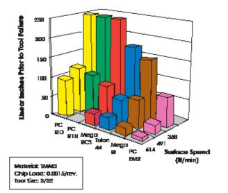
Figure #3 Ultimate Tool Life as a Function of Tool Size
