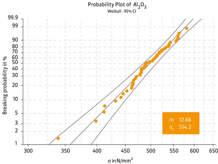
Diagram 1: Graphical description of a Weibull distribution with scale =  $\sigma_0$  for bending strength
