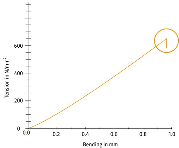
Diagram 2: tension vs. bending until break of sample
